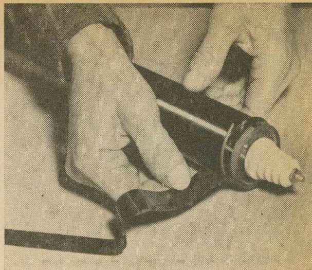
Fig. 14: Put the top disk in place and again, apply tape to finish, as you did on the bottom and overlap.
