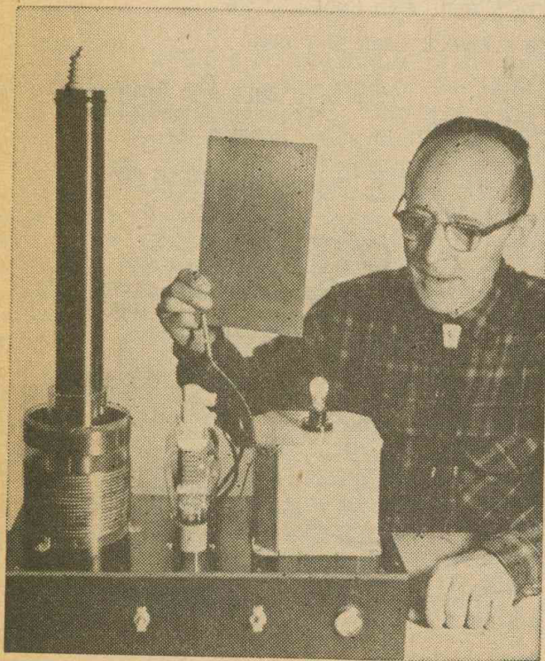
Fig. 6: A sheet of aluminum held in the hand serves as an antenna and helps light a small incandescent lamp.
